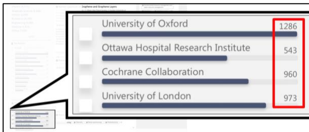
Figure 7. The filtering widget originally included a counts column (right). The team decided that task-motivated users like Abi might not see it as a filtering device, since it looks more like statistics. Team O removed it.
